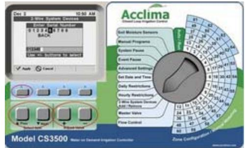
5. Repeat 1 through 4, entering serial numbers for all devices you have attached to the 2-wire system including valve adapters, sensors and flow meter modules.
