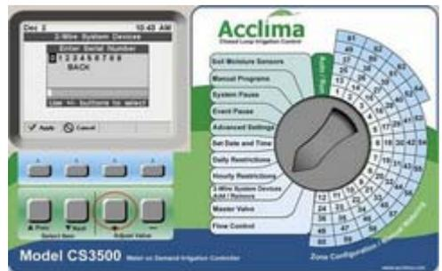
2. Use the Next/Prev keys to select the first digit of the serial number. Press + to enter the first
