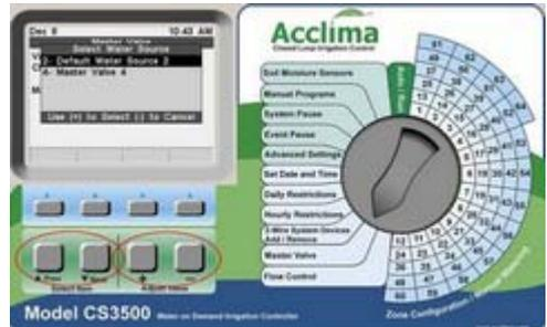
You can also test the valve current from this screen. Simply move to the Test Valve Current field using the Prev and Next Keys and press the adjust value button. This will take you to a test screen where you can test the valve current of just the master valve or all the system devices. (SEE TEST VALVE SCREEN)
