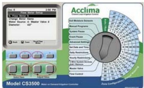
3. When you are finished with the flow meter settings press the soft Save key.
